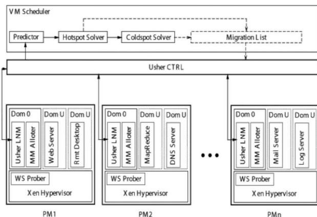
Virtual Machine Monitors (VMM) like Xen provide a mechanism for mapping Virtual Machines(VMs)
