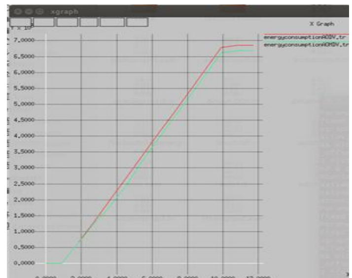
Fig7. Comparison of AODV and AOMDV energy consumption vs... Time
