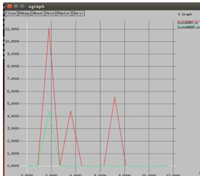
Fig 8: Comparison of AODV and AOMDV packet loss vs...Time
