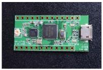
This Module is to connect the Mobile phone and RTK Module using OTG Cable
