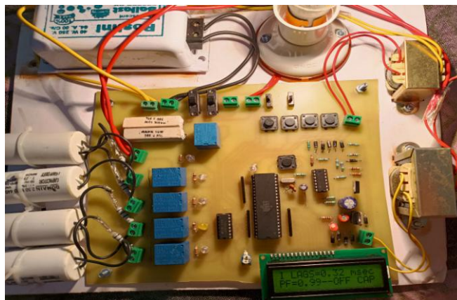
Fig. 3: When only Resistive Load is Present
